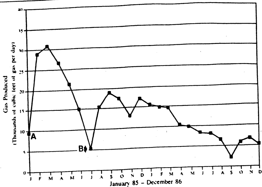
FIGURE 2 Gas and Oil Decline Curves for a Well in North Central Texas
